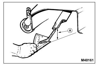
6. Measure from each outside blade tip (A) to the level surface. The difference between measurements must not be more than 3 mm (1/8 in).
